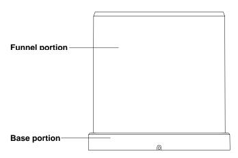
For accurate results, the rain sensor should be securely mounted onto a horizontal surface about 2-3ft above the ground and in an open area away from trees or other coverings where rainfall may be reduced causing inaccurate readings.
